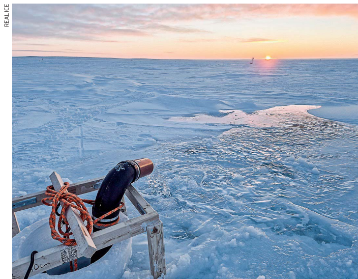
A pump delivers seawater to the surface of an ice sheet in Canada (above), and researchers measure the ice's thickness (below)
